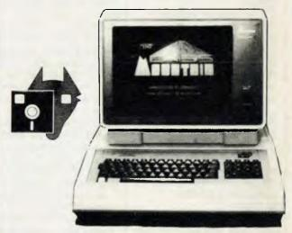
Complete with cooling fan, 13 preprogrammed keys, twin speakers, upper lower case, 64K, Forth card.
